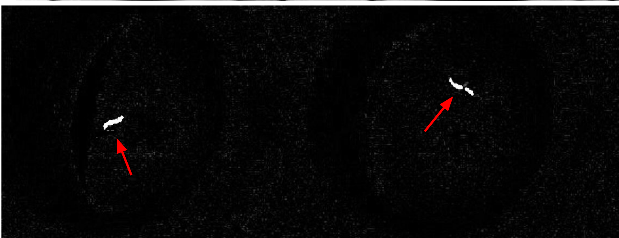
Count pixels that have changed in intensity to quantify movement
