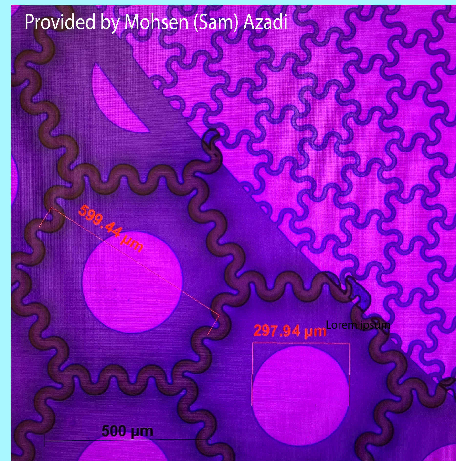
Figure 3. Spacer design and structure at three different microscale magnifications
