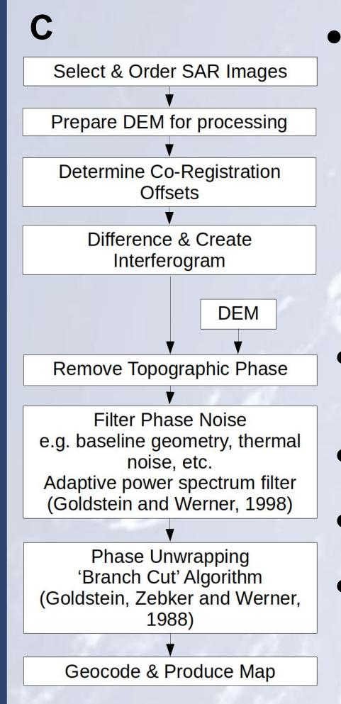
• (C): workflow for DInSAR processing using JPL/Caltech/Stanford InSAR Scientific Computing Environment (ISCE) package (Rosen et al., 2014).
