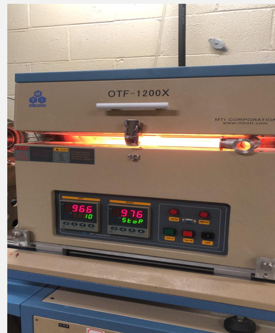
Image 3: Graphene 4" Furnace at 1000 degrees C
