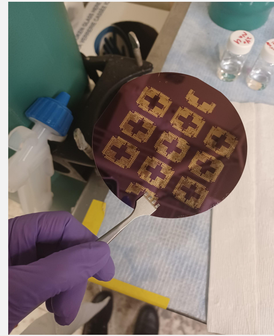
Image 4: Silicone Oxide Wafer with Au patterned GFET chips
