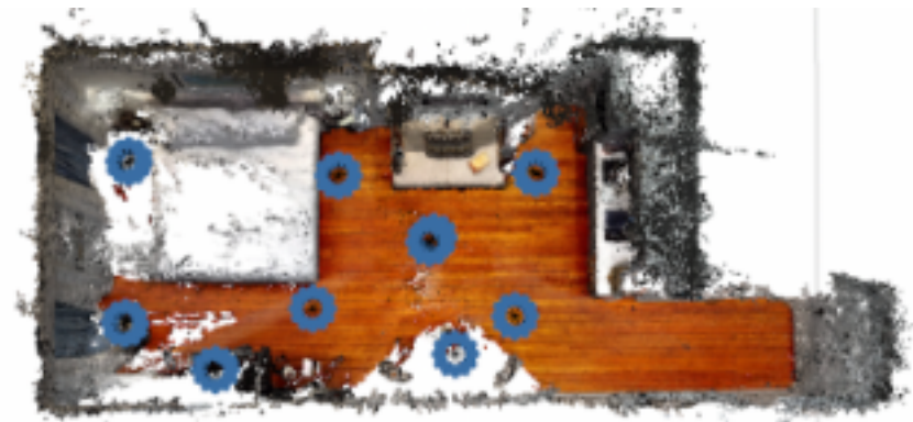
Figure. Dense-cloud 3D model recreated from Matterport Scanner data
