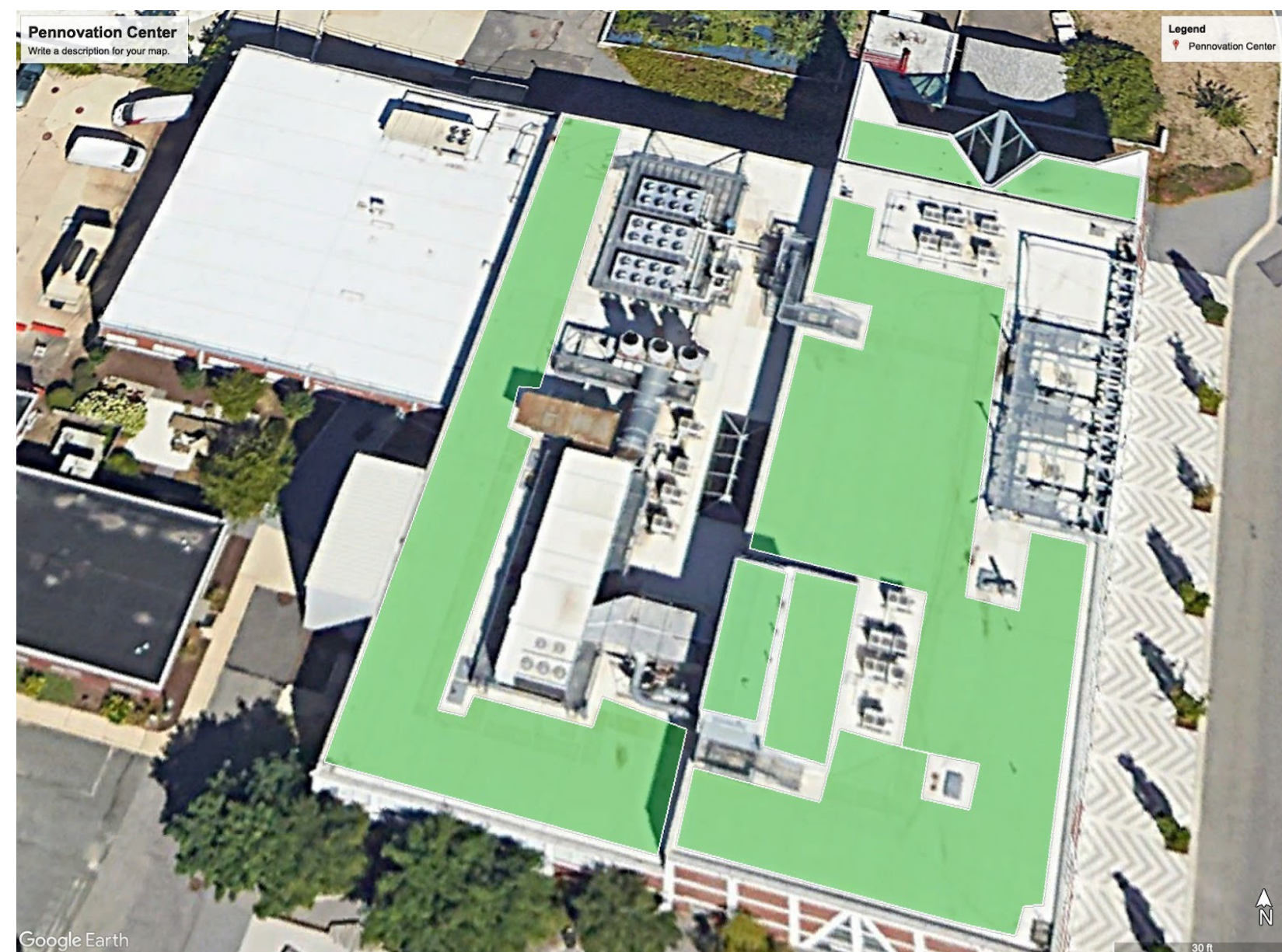
Figure 2: Where green and biosolar roofs could be placed, leaving service zones and buffers from the roof edge, highlighted in green (Google Earth Pro)
