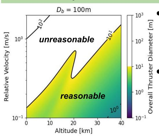
Main limiting factor: overall thruster diameter  $(D_{th})$  Also impacted by drag/buoyancy • Compensate for a few meters per second of wind velocity at ≤10 meters in overall diameter
