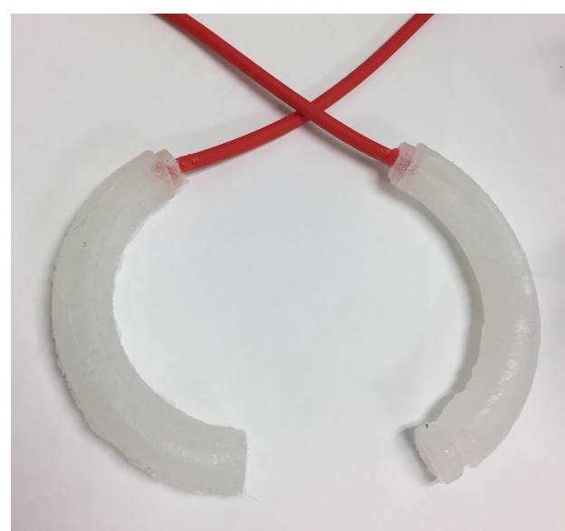
Fig 4. Silicone ring tube inside arms of toy to measure grasping forces
