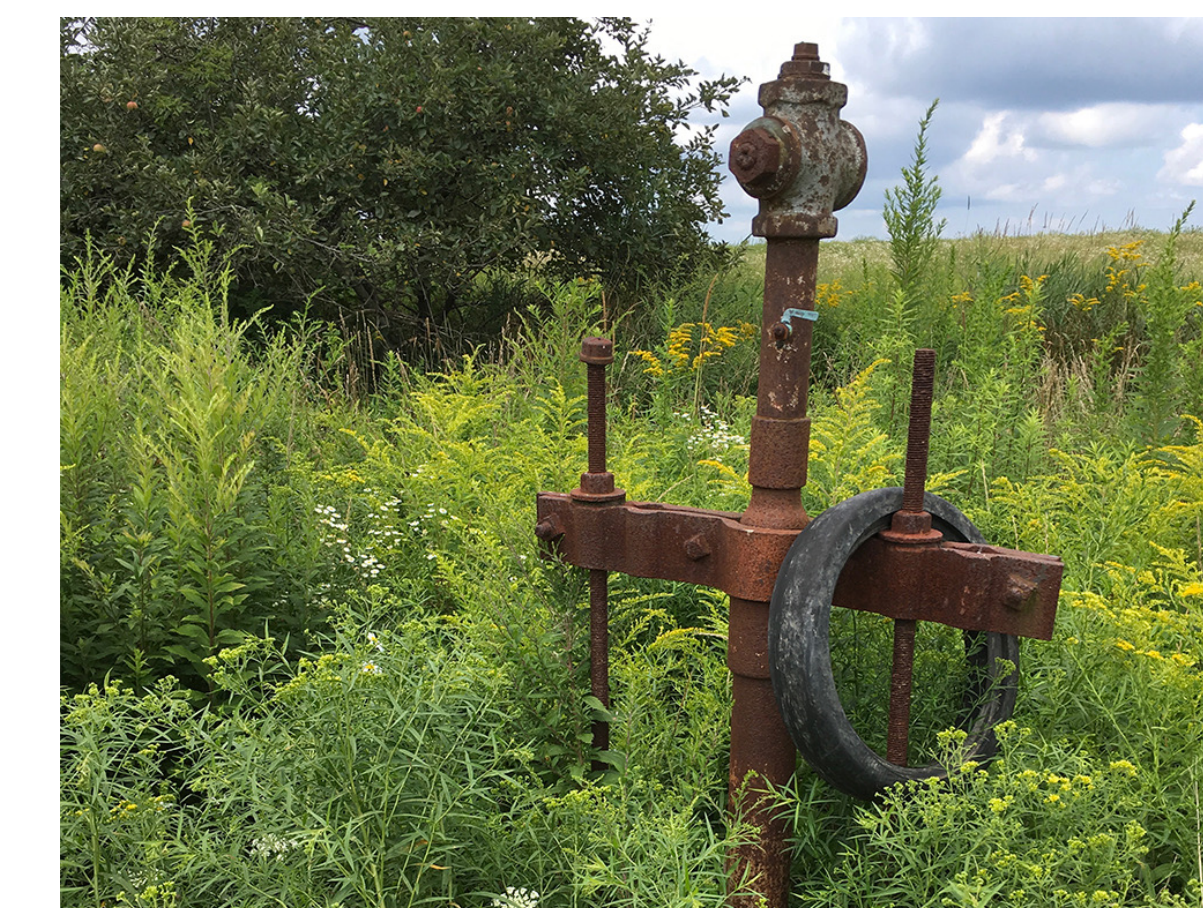
Image of plugged well from PA DEP
