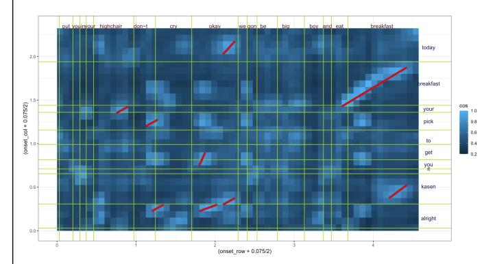
One utterance is on the x-axis and the other is on the y-axis. The first sound of the first utterance is compared to every sound of the second sentence. This is done for all sounds of both sentences. The stretches of light blue boxes mean that there was a stretch of time in which the sounds of both sentences were very similar.
